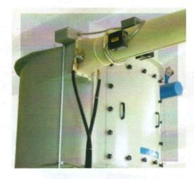
Fires that start in production machinery quickly spread to the air filtration system. If the air filtration system is disabled by fire damage, a mill cannot continue to operate its production machinery.
