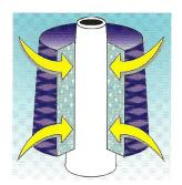
Homogeneous penetration of moisture is ensured by several stages of evacuation and impregnation with saturated steam. Precision sensors with perfect reproduction system ensures consistent performance within and between batches for years of operation.
